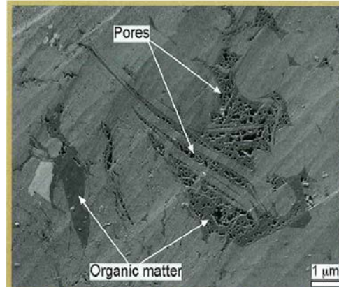
Figure 3. Field emission scanning electron photomicrograph of nanoscale pore architecture in the Barnett Formation. Image provided by R. Reed.
